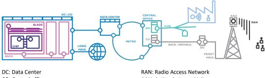
CO: Central office DU: Distribution Unit RAN: Radio Access Network AAU: Active Antenna Unit PON: Passive Optical Network
