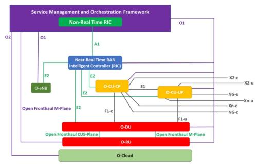
Figure 13: RAN overall logic architecture with O-RAN specific interfaces depicted in green [ORA19].
