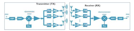
Figure 17: Beamforming in a wireless transceiver (PLL: phase-locked loop, LNA: low-noise amplifier, PA: power amplifier, ADC: analog-to-digital converter, DAC: digital-to-analog converter, DSP: digital signal processing, Δφ: phase shifter).
